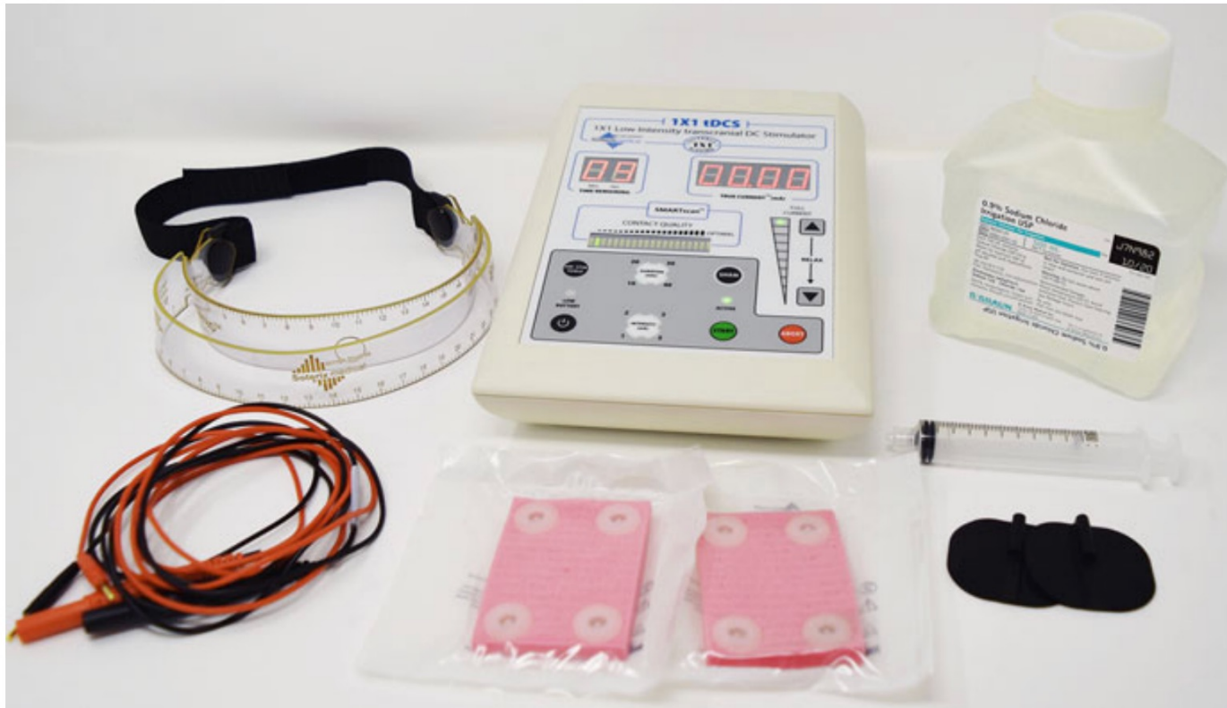
Fig. 1 Example of a tES device and a headgear used for electrical stimulation with sponge electrodes. In general, conventional sponges are soaked with a controlled volume of saline using a syringe. Rubber electrodes (electrochemical electrodes) are placed inside the sponge pockets. Lead wires connect to the device to the conductive rubber electrodes. Sponge electrodes are then secured on the scalp using a headgear. The rubber electrodes inside the saline-soaked sponge pockets are energized using a corresponding lead wire connected to the device
