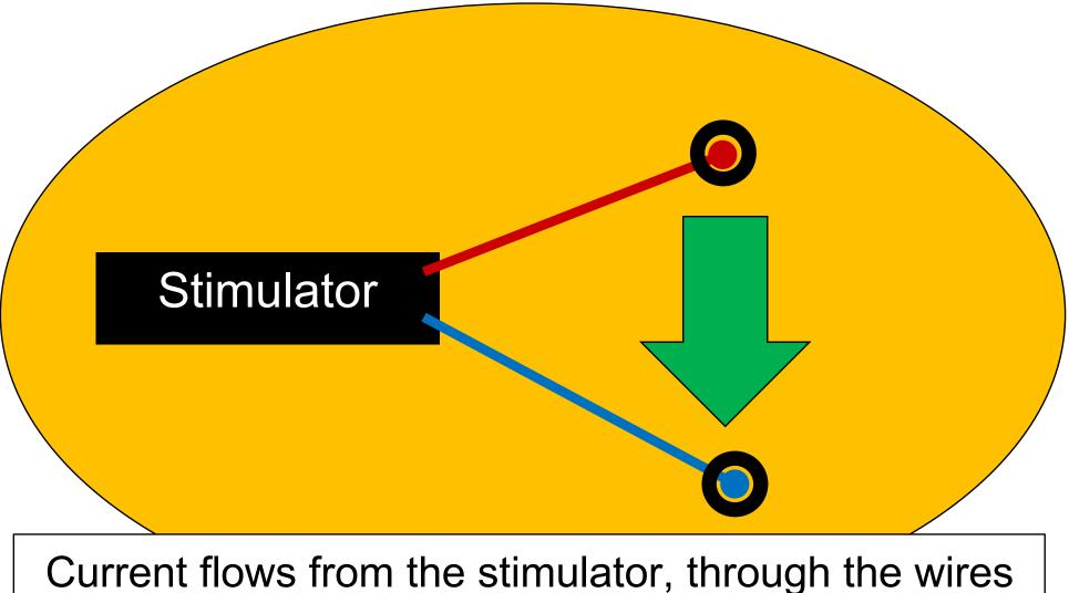
(leads) and to exposed metal contacts (Electrodes)
