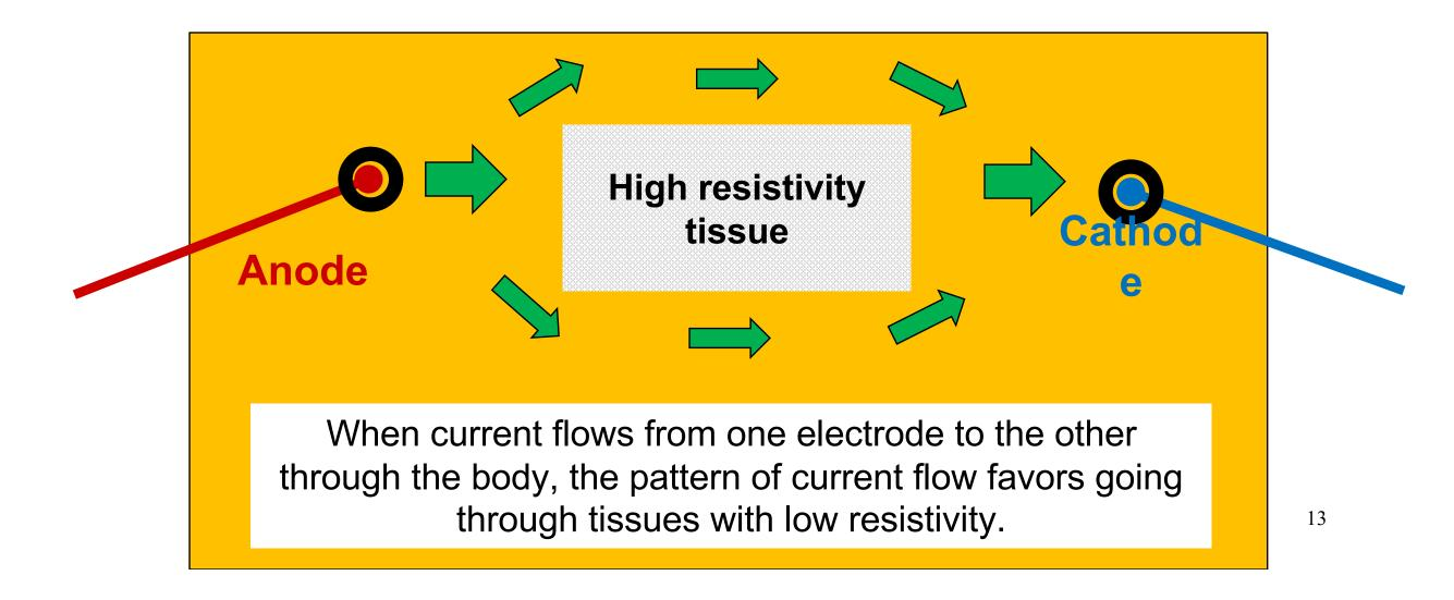
Details of body anatomy and associated tissue **resistivity** can lead to **current patterns** that are hard to guess.
