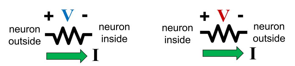
The idea of current flowing into the neurons **hyperpolarizing** and current flowing out of the membrane **depolarizing** extends to more realistic neurons shapes.
